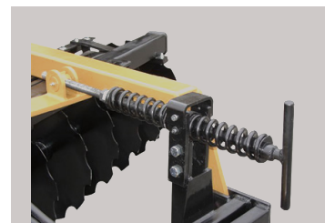
Self-leveling spring cushioned with hand crank
