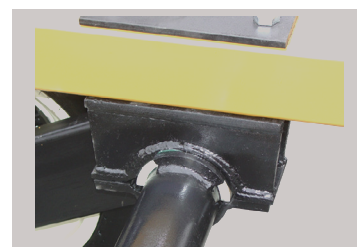
Replaceable nylon bearings on wheel mounts
